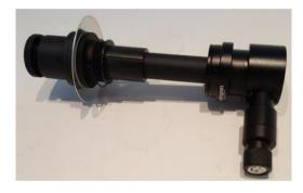
To do this, the polarscope must be inserted at the rear end, i.e. the area with the three grub screws. Before doing this, make sure that the grub screws do not protrude into the socket of the additional lighting device. Then tighten the grub screws very slightly without exerting pressure, as this is perfectly sufficient to ensure a secure grip.
